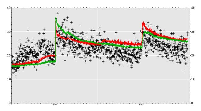
Figure 7.5 A comparison of hourly data from the CRNS (black), with 30 minute data from two TDT sensors (red and green). [Note that changes in processing may mean that this plot does not reflect currently available data.]
