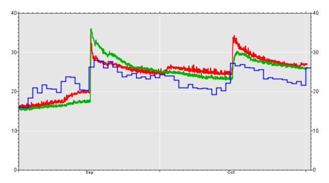
Figure 7.6 A comparison daily VWC data from the CRNS (blue) with 30 minute data from the two TDTs (red and green). [Note that changes in processing may mean that this plot does not reflect currently available data.]
