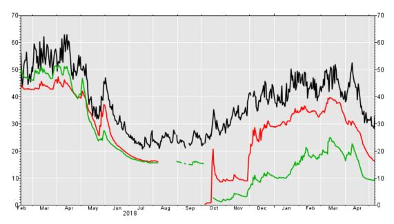
Figure I.1 Soil moisture (VWC %) from the CRNS (black), TDT1 (red) and TDT2 (green) showing the dramatic effect of instrument swap.
