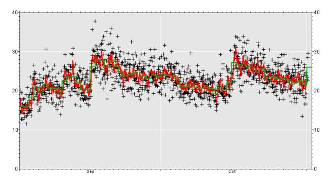
Figure 7.4 A comparison of VWC data from the CRNS: hourly (black), 7-hour moving average (red) and daily (green). [Note that changes in processing may mean that this plot does not reflect currently available data.]
