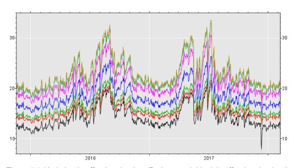
Figure 7.3 Variation in effective depth at Rothamsted: black is effective depth others are D86 from top to bottom at 1m (brown), 5m (cyan), 25m (pink), 75m (blue), 150m (green) and 200m (red) from the sensor. [Note that changes in processing may mean that this plot does not reflect currently available data.]
