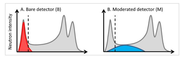
Figure 7.2 Sampling of neutron energy spectra by bare and moderated detectors, from Andreasen et al. (2016). The dashed line represents 0.5eV.
