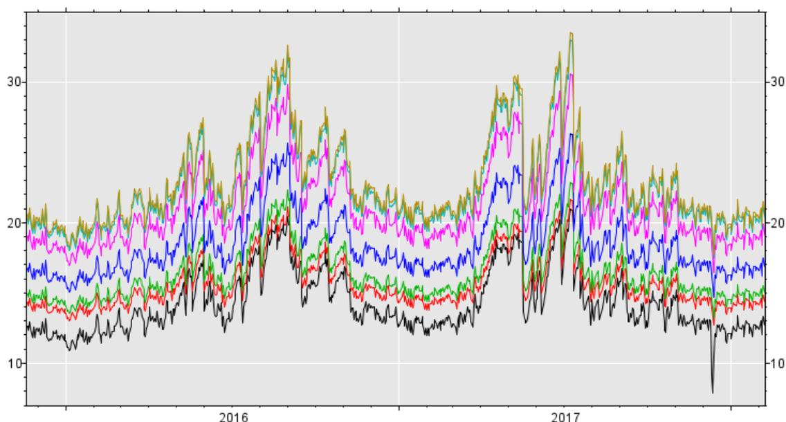
*Figure 7.3 Variation in effective depth at Rothamsted: black is effective depth others are D86 from top to bottom at 1m (brown), 5m (cyan), 25m (pink), 75m (blue), 150m (green) and 200m (red) from the sensor. [Note that changes in processing may mean that this plot does not reflect currently available data.]*
