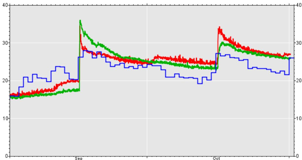
*Figure 7.6 A comparison daily VWC data from the CRNS (blue) with 30 minute data from the two TDTs (red and green). [Note that changes in processing may mean that this plot does not reflect currently available data.]*
