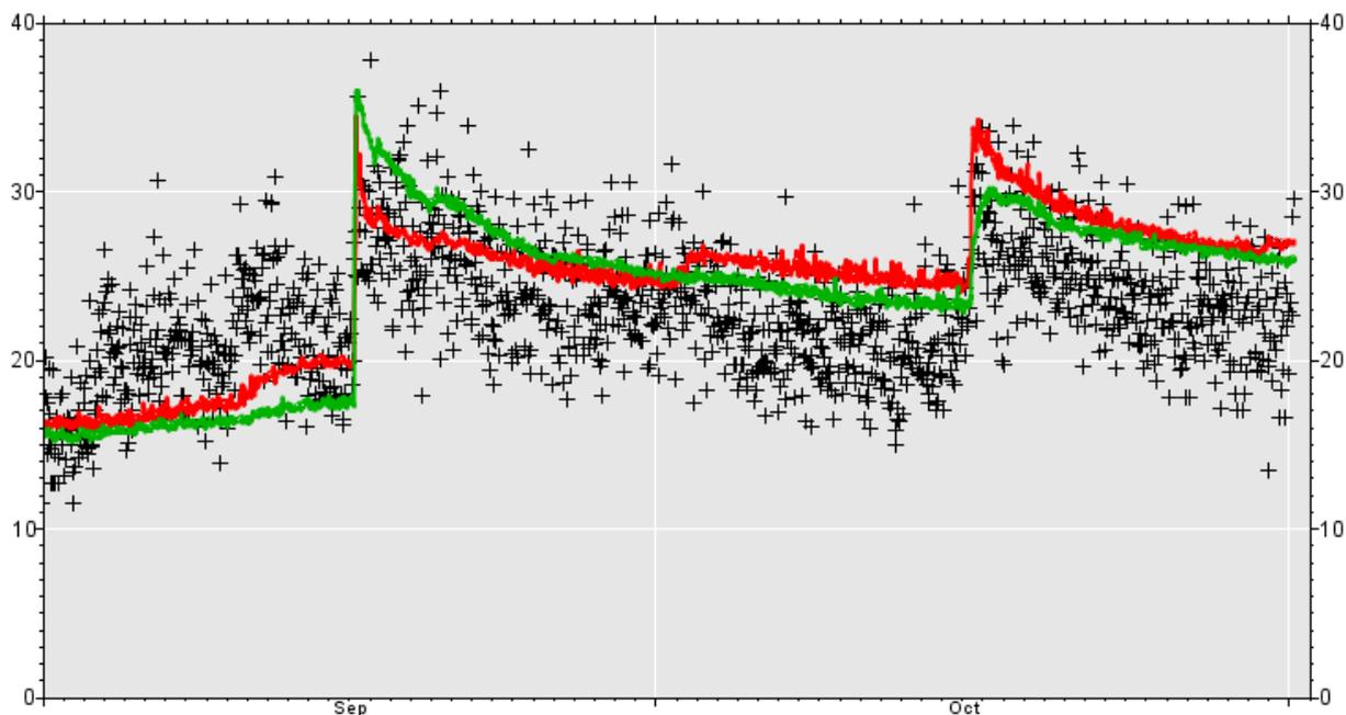
*Figure 7.5 A comparison of hourly data from the CRNS (black), with 30 minute data from two TDT sensors (red and green). [Note that changes in processing may mean that this plot does not reflect currently available data.]*
