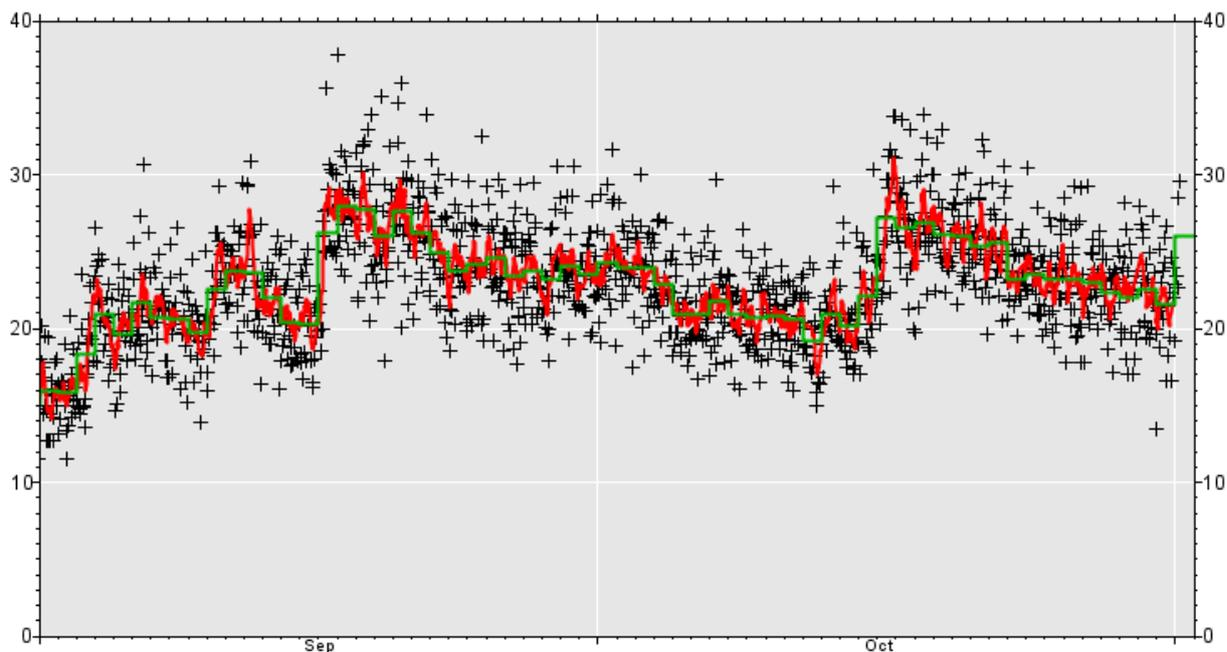
*Figure 7.4 A comparison of VWC data from the CRNS: hourly (black), 7-hour moving average (red) and daily (green). [Note that changes in processing may mean that this plot does not reflect currently available data.]*
