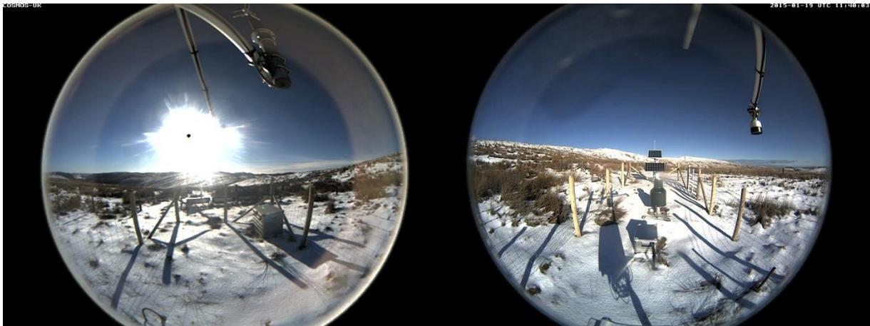
*Figure C.2 Snow as recorded by the phenocam at Plynlimon. Note also the burning on the south facing image on the left caused by the camera pointing directly at the sun on a clear day.*
